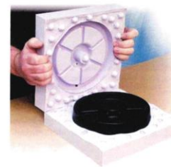
Silicone rubber mold and cast urethane part, courtesy Reynolds Advanced Materials
