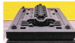
3D-printed sand core for a large metal casting, courtesy of ExOne
