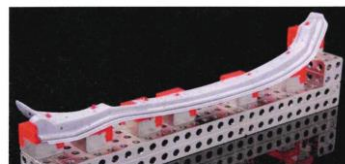
Materialise RapidFit custom holding fixture for inspection (parts in orange made by AM), courtesy of Witte Barskamp KG
