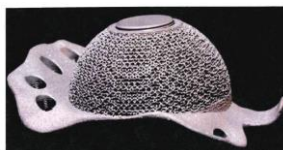
Patient-matched acetabular cup made in titanium by AM for a patient needing revision surgery (note porous and solid regions constructed as a single part), courtesy of Osia Ltd.
