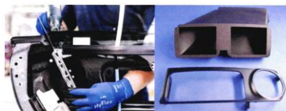
Window guide rail (left), courtesy of BMW; air duct (top, right) and part for heating control unit (bottom, right) made in PA12 by laser sintering, courtesy of Daimler
