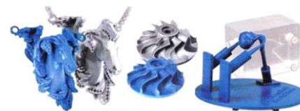
AM-produced investment casting patterns (blue) and finished cast metal parts, courtesy of 3D Print Color
